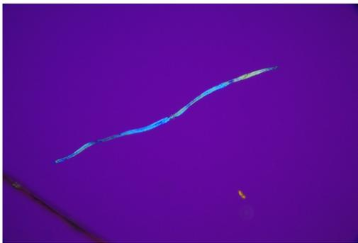
(c) Paper fibre with the gypsum plate inserted
