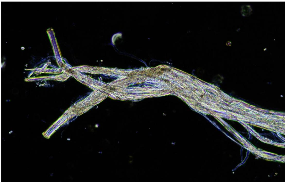
(b) In dispersion staining the fibres look white. In this case the asbestos is chrysotile in a liquid with a R.I of 1.6700. Taken with 125x magnification.
