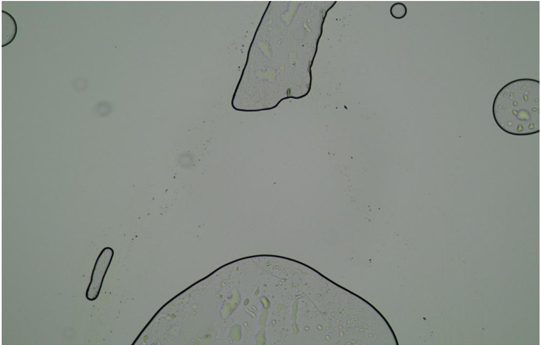
(a) Chrysotile in plane-polarized light. The chrysotile fibres are barely seen as they are in a liquid with the same refractive index. Taken with 125x magnification.
