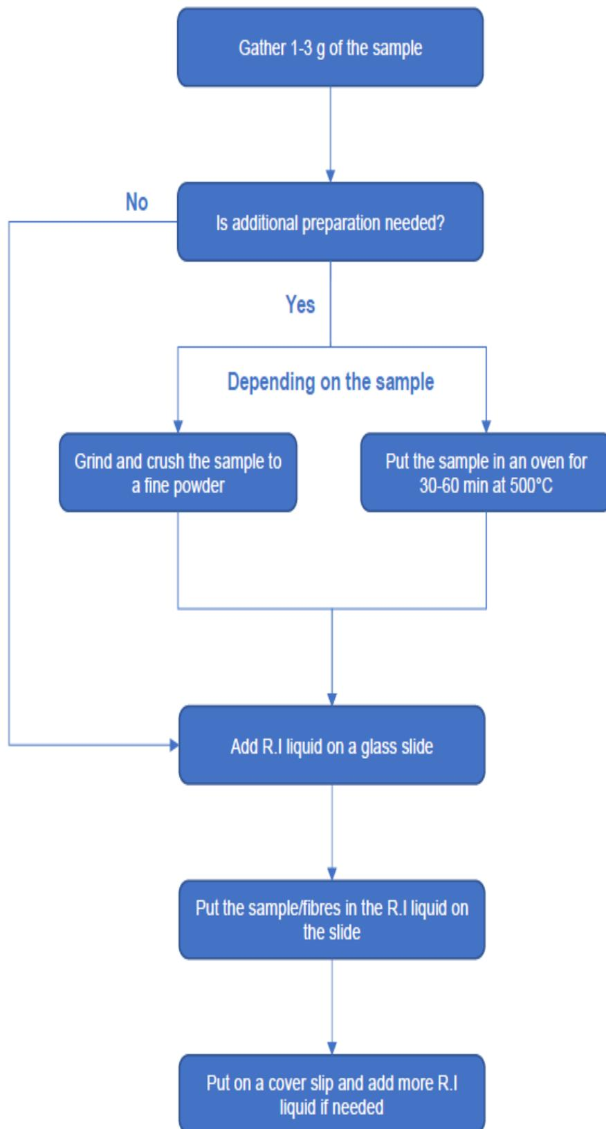
Figure 6: A simple overview of the steps required for sample preparation for the PLM method.
