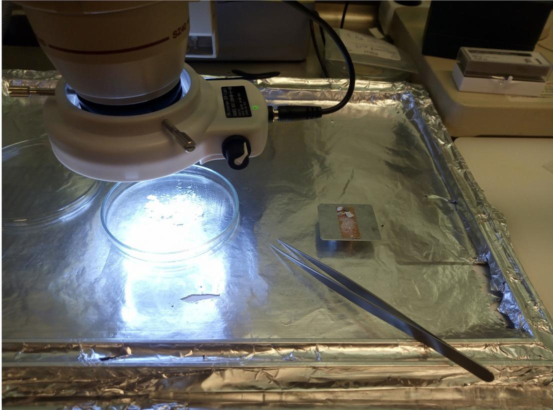
**Figure 8:** For the SEM-EDS method the prepared samples are added to a copper tape.
