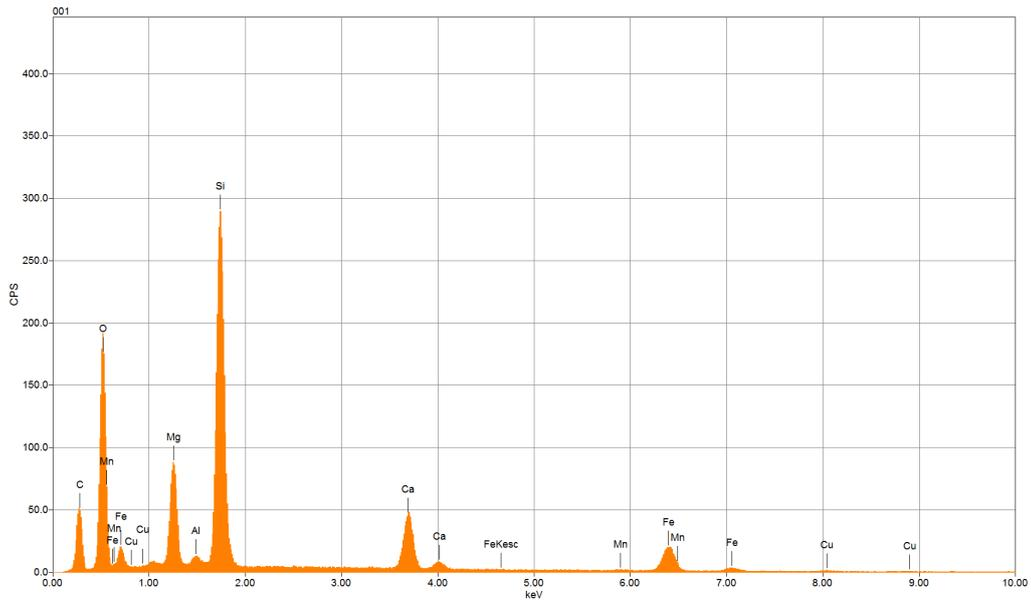
(a) Actinolite asbestos:  $Ca_2(Mg,Fe)_5Si_8O_{22}(OH)_2$
