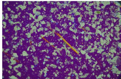
(b) Wollastonite in cross-polarized light with gypsum plate inserted
