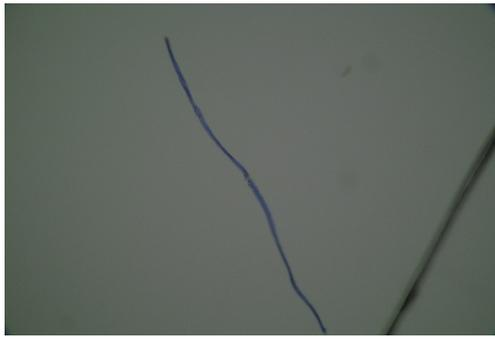
(a) Paper fibre in plane-polarized light
