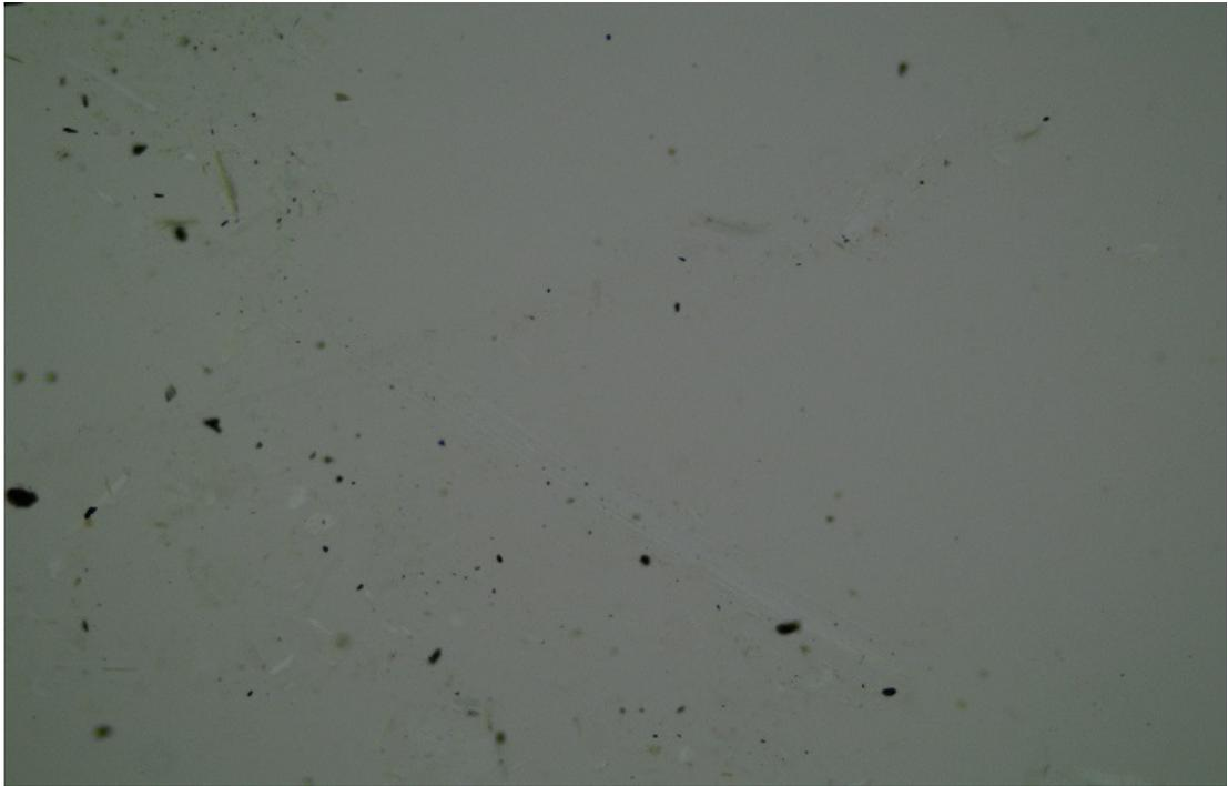
(a) Anthophyllite asbestos fibres are almost invisible in plane-polarized light when in the correct R.I. Taken with 125x magnification.
