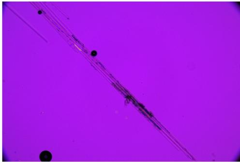
(c) Glass fibres in cross-polarized light with the gypsum plate inserted
