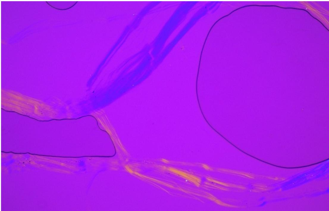
(d) When the fibre is rotated 90° degrees the colour changes. The easiest way to find asbestos fibres in the sample is with cross-polarized light with the gypsum plate inserted. Taken with 125x magnification.
