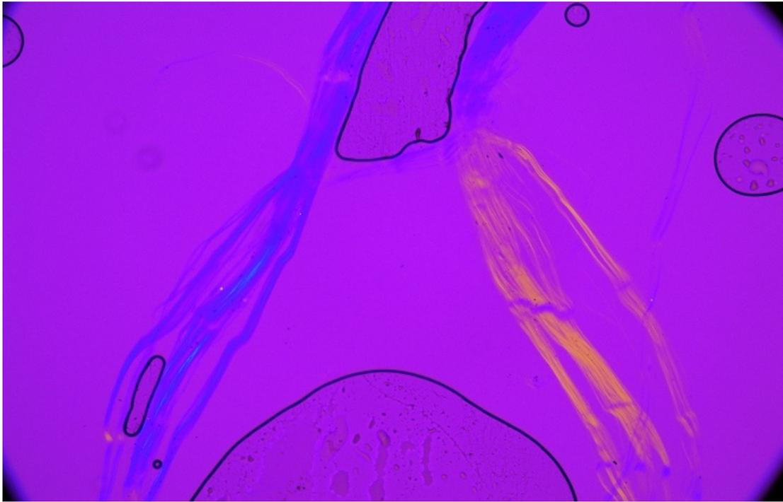
(c) When the gypsum plate is inserted in cross-polarized light the fibres show the sign of elongation. All asbestos fibres except crocidolite have the same sign of elongation. Taken with 125x magnification.
