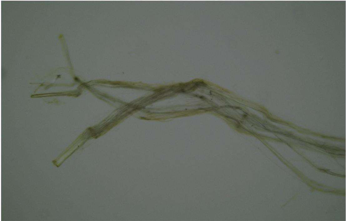
(a) When an asbestos fibre is in the wrong R.I it can clearly be seen in plane-polarized light. Taken with 125x magnification.
