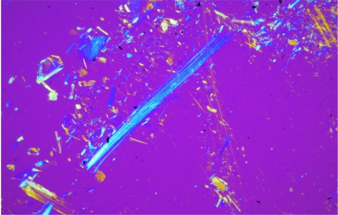
(c) Asbestos fibres show clear colours in cross-polarized light with the gypsum plate inserted. This shows the sign of elongation. Taken with 125x magnification.
