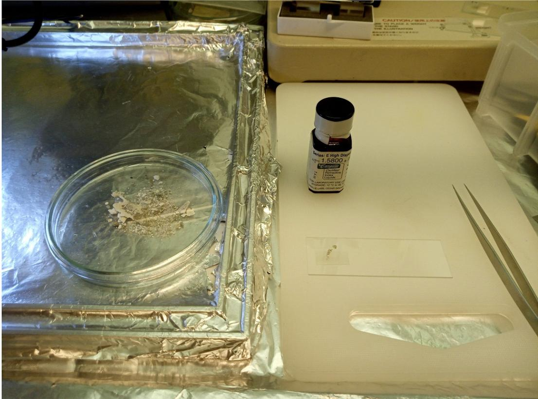
**Figure 7:** The prepared samples are added to a glass slide that has a drop of R.I liquid. The R.I liquid is chosen based on suspected asbestos type or if none are suspected the 1.5800 liquid is used.
