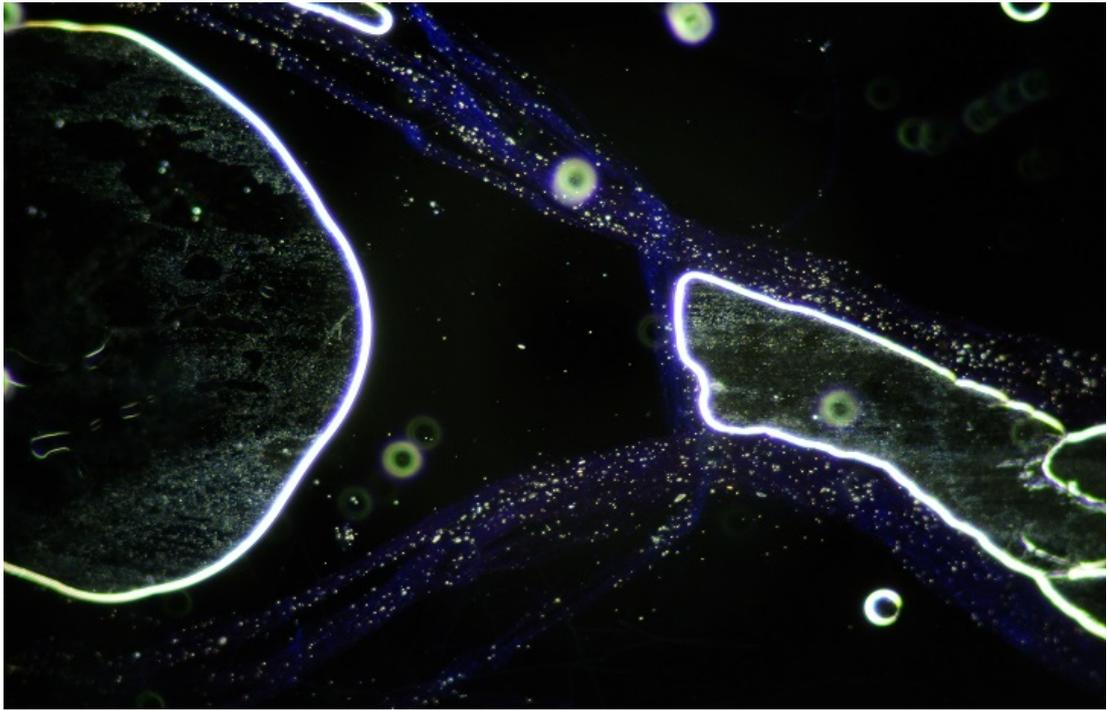
(e) When chrysotile is in the correct R.I it shows blue-magenta colours in dispersion staining. Taken with 125x magnification.
