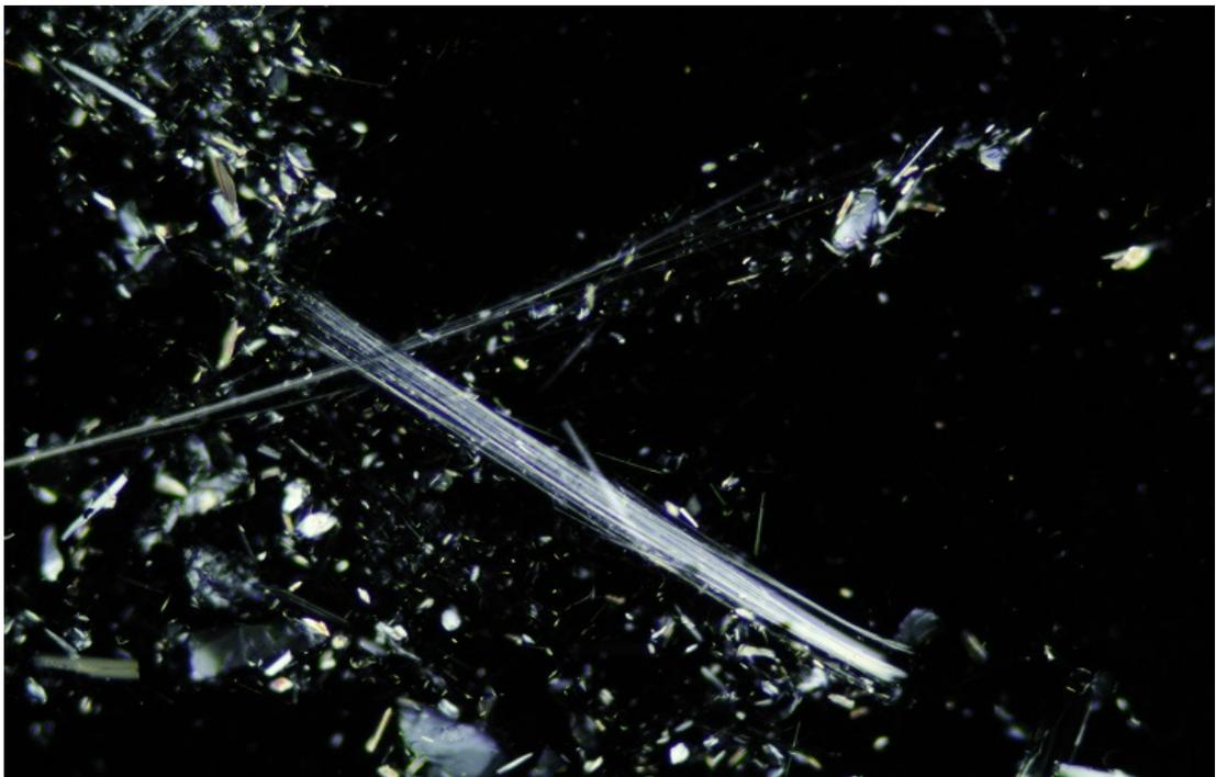
(b) When viewed in cross-polarized light the fibres are clearly visible. The fibres show even colouration typical for mineral fibres. Taken with 125x magnification.
