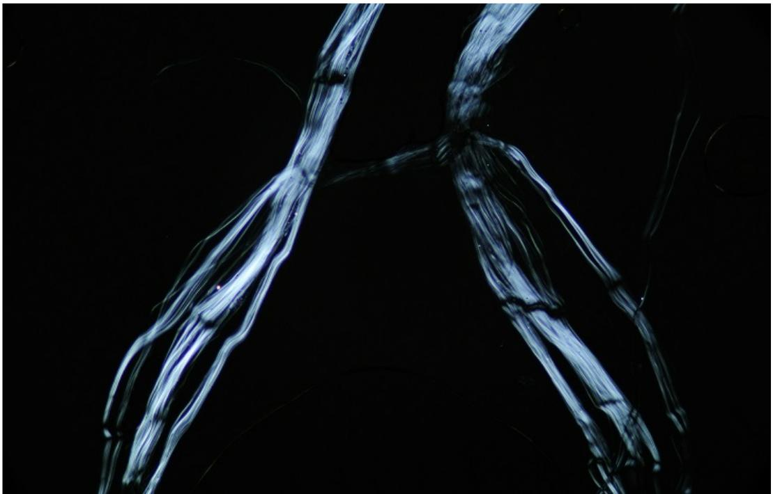
(b) In cross-polarized light the same chrysotile fibres are clearly visible. They also show an even colouring that is only seen in mineral fibres. Taken with 125x magnification.
