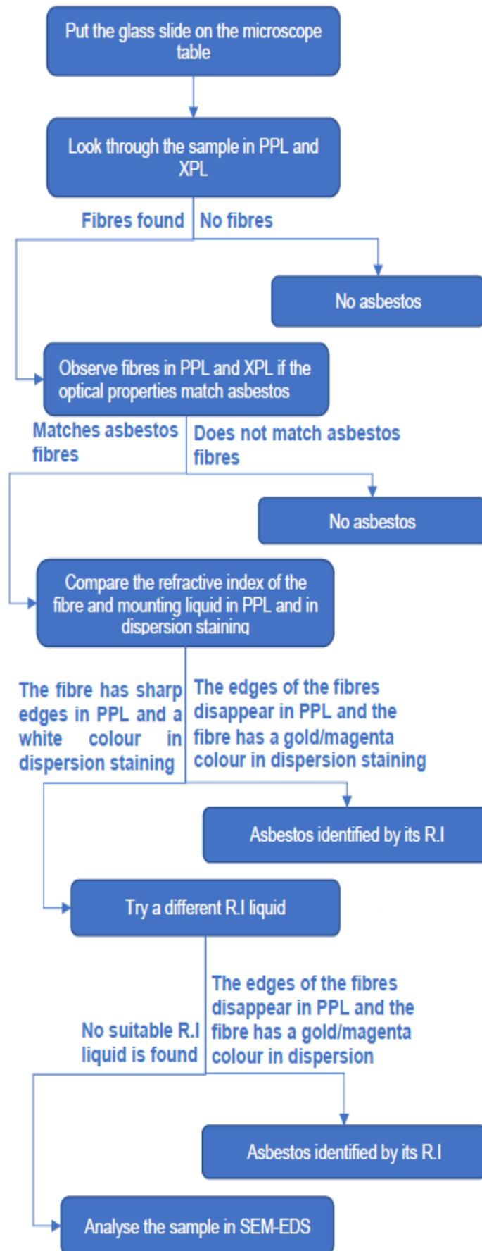
Figure 10: A flowchart of the steps done to identify asbestos with the PLM method.
